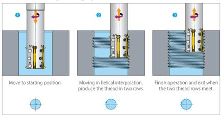
MiTM Offset inserts come in two different sizes - 25mm (MiTM25) & 41mm (MiTM41). Additionally, each insert offers two cutting edges per insert.
